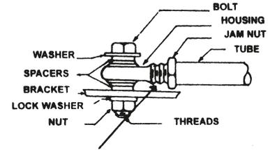
**IMPORTANT:** If a 3/4 inch rod end is used, there should be no more than 3/4 inch of thread showing on shank of rod end. Sample applies to 1/2" and 5/8" rod ends. Size of rod ends dictates length of thread showing.
